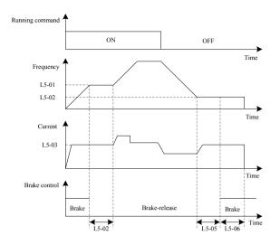
Fig.5-30 Band-type braking control process illustration
