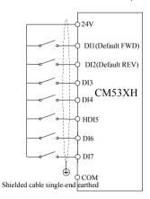
DI terminal connection Mode 2: DI dial switch in NPN mode and with external power supply
