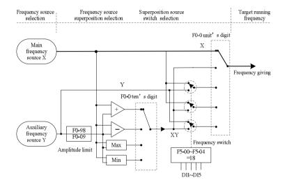
Fig.5-1 Illustration of frequency source superposition
