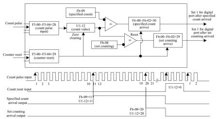
Fig.4-25 Counting mode function code setting
