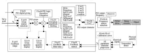
Fig.4-19 Illustration of frequency closed loop control
