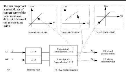
Fig.4-28 The actual given of AI signal
