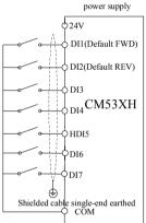
DI terminal connection Mode 1 (Default) : DI dial switch in NPN mode and without external
