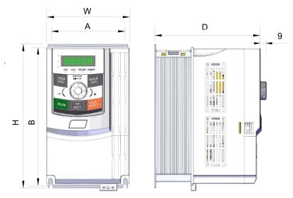
Fig.2-4 Installation dimensions of plastic mode below 7.5 KW
