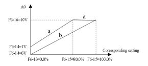
Fig.5-12 Analog output limitation corresponding relationship
