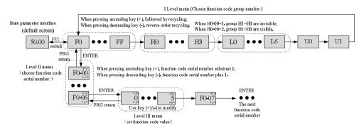
Fig.4-3 three-level menu operation flow chart
