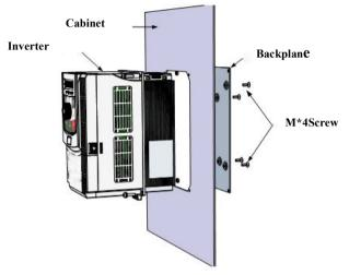
Fig.3-3. CM53XH Wall-mounted installation instruction of plastic structure
