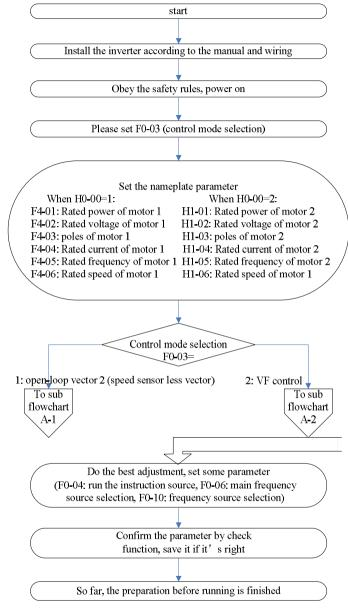
Figure 4-6 basic steps before running
