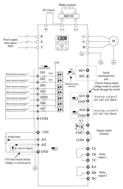
Fig.3-9 three-phase inverter above 75KW
