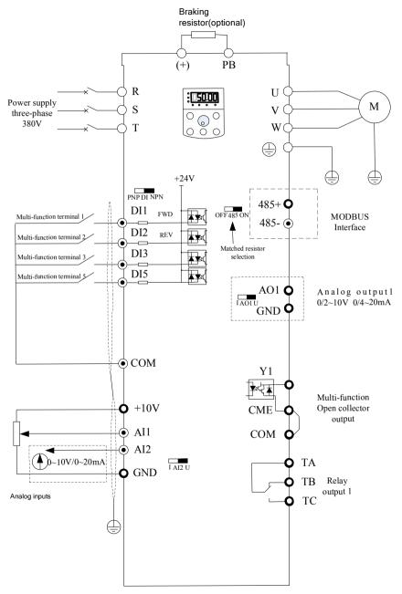
Fig.3-6 three-phase inverter under 1.5KW
