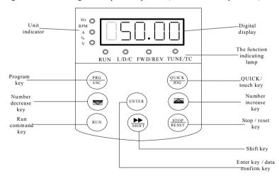
Fig.4-2 Schematic diagram of operation panel 2
