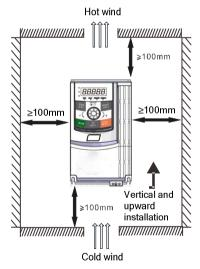
Fig.3-1 single one installation illustration
