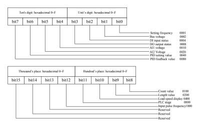
Fig.5-8 LED stop display illustration
