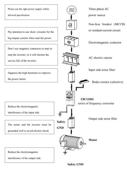
Fig.1 illustration of connecting to the peripheral machines
