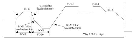
Fig.5-27 simple PLC illustration
