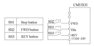
Fig.5-9 Three wire control mode 1
