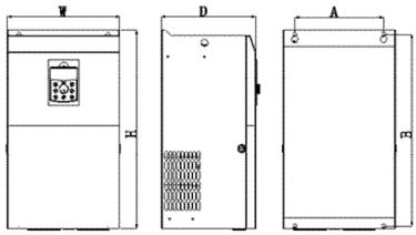
Fig.2-6 appearance and install dimension of inverter within 45KW~132KW
