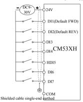
DI terminal connection Mode 4: DI dial switch in PNP mode and with external power supply
