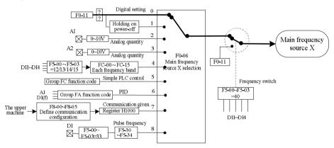
Fig.4-17 Illustration of main frequency source setting
