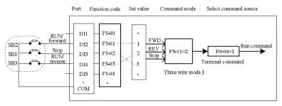
Fig.4-10 Illustration of terminal control start-stop mode
