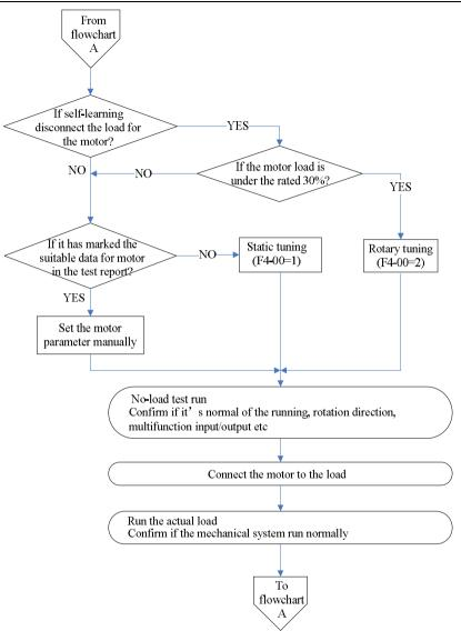
Fig.4-7 open-loop vector control running steps
