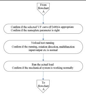
Fig.4-8 V/F control mode running steps
