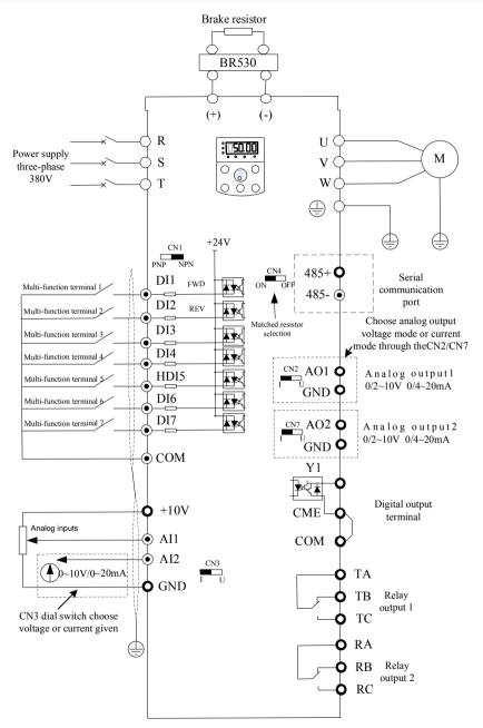
Fig.3-8 three-phase inverter within 30KW~55KW
