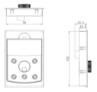
Fig.2-7 outer keyboard with plate installation dimension
