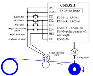
Fig. 4-24 Examples of fixed-length control function
