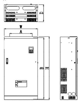
Fig2-7 Installation dimensions of metal mode above160KW
