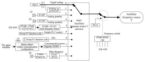
Fig.4-18 Illustration of auxiliary frequency source setting
