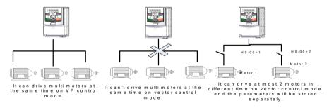
Fig.4-26 Switching of multi-group motors
