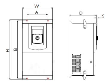
Fig2-5 Installation dimensions of metal mode within 11~37KW
