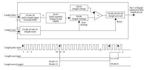
Fig.4-23 Function code setting of fixed-length control mode
