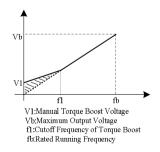
Fig.5-4 Illustration of Manual Torque Boost
