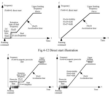
Fig.4-13 Pre-excited magnetism start illustration
