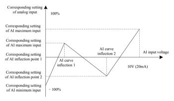
Fig.5-29 Multi-point corresponding illustration
