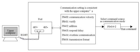
Fig.4-11 Illustration of communication control start-stop mode
