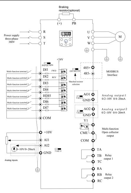
Fig.3-7 three-phase inverter under 22KW
