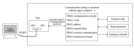
Fig.4-30 communication setting illustration
