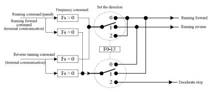
Fig.4-22 Illustration of motor running direction
