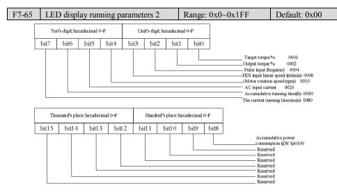
Fig.5-20 LED running display illustration
