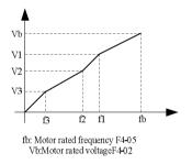
Fig.5-5 schematic diagram for V/F curve setup
