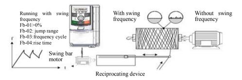
Fig.4-20 Illustration of swing frequency application setting
