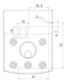
Fig.2-8 outer keyboard without plate installation dimension
