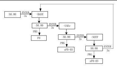
Fig.4-5 operation diagram of the menu mode switch
