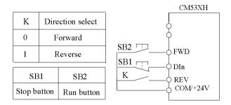
Fig.5-10 Three wire control mode 2
