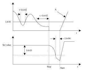
Fig.5-31 Sleep process frequency illustration
