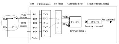
Fig.4-9 Illustration of terminal control start-stop mode
