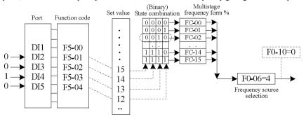
Fig.4-21 Illustration of multi-speed control mode
