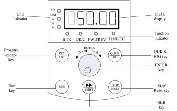
Fig.4-1 schematic diagram of operation panel 1 (standard LED keyboard 1)
