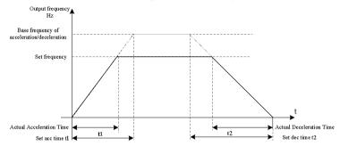
Fig.5-2 Illustration of acceleration/ deceleration time
